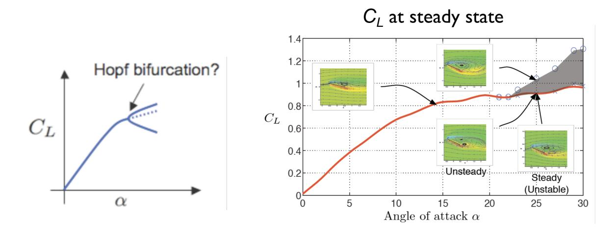
Are there high-lift unstable steady states in low aspect ratio airfoils?
