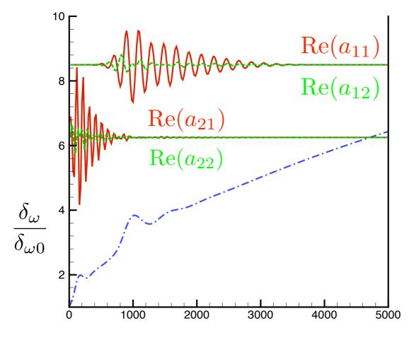
Thickness and amplitude of POD modes for k=2 initial condition: low-dimensional model
