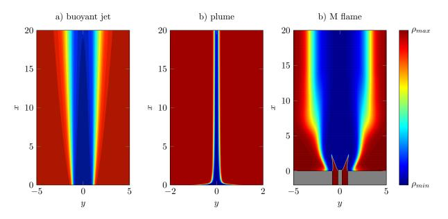
FIGURE 1. Density distributions in the meridional plane of axisymmetric base flows. Lengths are scaled with the radius of the inlet orifice. a) Jet at Re = 200 and  $Ri = 10^{-4}$ ; b) plume at Re = 200 and  $Ri = 10^3$ ; c) premixed *M*-flame at Re = 950 and  $Ri = 1.6 \times 10^{-4}$ .
