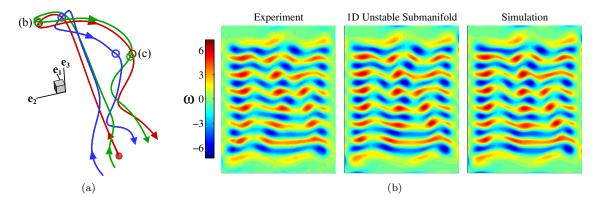
Figure 1: (a) A projection showing an unstable equilibrium (red sphere) with the dominant unstable submanifold (red curve). Experimental (blue curve) and numerical (green curve) turbulent trajectories follow this submanifold as they depart from the neighborhood of the unstable equilibrium. (b) Representative flow fields from the submanifold and two turbulent trajectories (denoted with circles in (a)).
