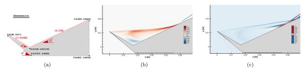
Figure 2: (a) Tick geometry. Amplitude functions of least-damped linear global mode; (b)  $\hat{u}$  and (c)  $\hat{p}$ .
