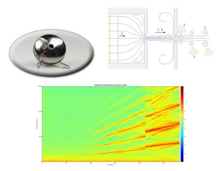
FIGURE 1. (a) : Birdall used in this work. (b) sketch of the flow (according to [?]). (c) time-frequency diagram.
