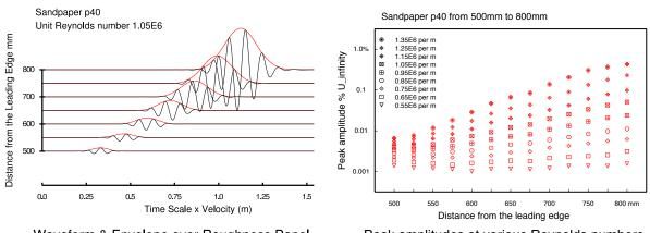
Waveform & Envelope over Roughness Panel
