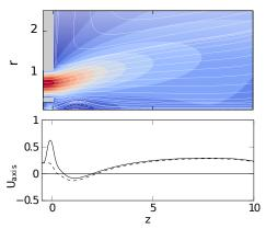
FIGURE 1. Controlled flow field and comparison between the velocity on the axis of the uncontrolled (dashed) and controlled system.
