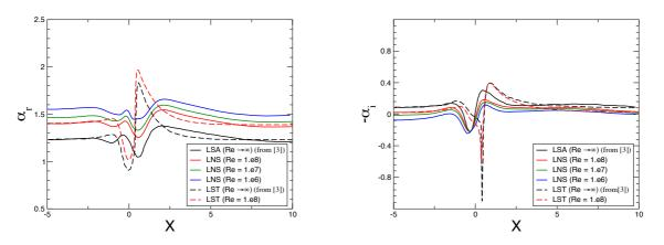
FIGURE 1. Wavenumber  $\alpha_r$  (left) and growth rate  $-\alpha_i$  (right) of a TS wave at frequency  $\omega = 3.0$  for a hump with height h=2.0 and width d=0.5 located at X = 0.0 on a flat plate.
