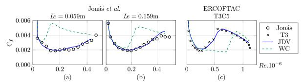
FIGURE 1. Skin friction coefficient for 2 of the 6 cases from Jonáš et al. [7] (Tu = 3% with different integral length scales Le) and for the ERCOFTAC T3C5 case, with adverse pressure gradient.
