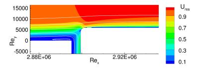
FIGURE 2. Base flow for  $Re_h = 6\,000$  and rounded step, strong suction.
