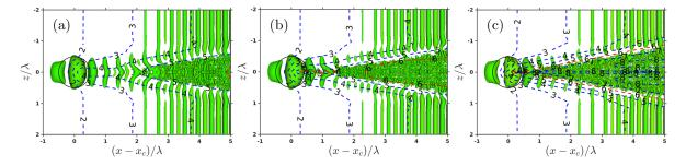
FIGURE 1. Comparison of laminar-turbulent transition onsets for different h in a large domain. The parameter  $\lambda = 81$ mm. (a) h = 1.620mm; (b) h = 1.895mm; (c) h = 2.170mm. The iso-surfaces are generated by pressure fields. The red dashed lines indicate the contour lines with the transition criteria N-factor 6. The solid circles indicate the indentation boundaries  $r = \lambda/2$ .
