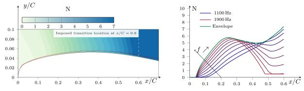
FIGURE 1. N-factor extraction on an ONERAD (symmetrical) airfoil in 2D subsonic conditions.
