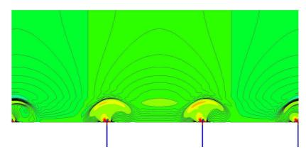
FIGURE 1. interaction of a temporally growing TS-wave (contour-lines) with acoustic perturbations (color-coded wall-normal velocity) emitted from three suction-slots.
