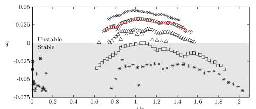
FIGURE 2. Eigenvalue spectrum for different lengths of the domain,  $460\delta_0^*$  (×),  $390\delta_0^*$  (°),  $320\delta_0^*$  ( $\Delta$ ),  $250\delta_0^*$  ( $\Box$ ),  $180\delta_0^*$  (\*), where  $\delta_0^*$  refers to the displacement thickness at the inlet.
