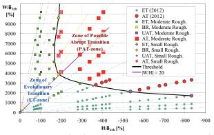
FIGURE 1. Zones of Evolutionary Transition (ET) and Possible Abrupt Transition (PAT) in plane of dimensionless values of gap depth and gap width for all cases studied in the present work. Inclined lines display constant aspect ratios |W/H| in a range from 0.5 to 100.
