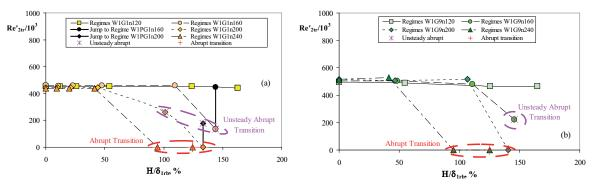
FIGURE 1. Transitional Reynolds numbers versus dimensionless roughness height obtained for various freestream speeds for elevated Tu-levels generated by grids G1 (a) and G9 (b) for roughness-strip width of 50 mm (case W1).
