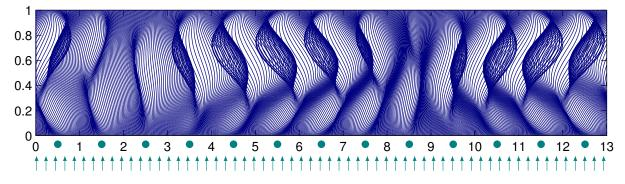
FIGURE 1. Streaklines (in the x-y-plane) of a wake past 13 cylinders. Visualized is the second least stable mode, showing a synchronization of individual units.
