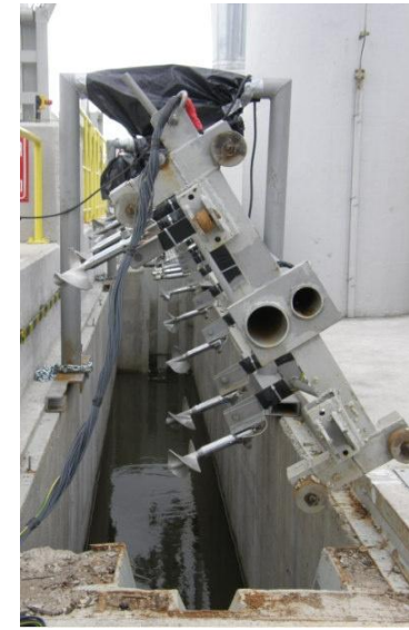
Installation of the current meters for cam-curve determination
