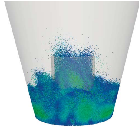
Figure 4: Numerical simulation based on coupled CFD-DEM for a Wurster type fluidised bed coater
