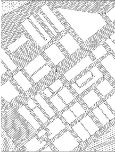
Figure 10: A section of the polyhedral mesh topology at the ground surface of the computational domain.
